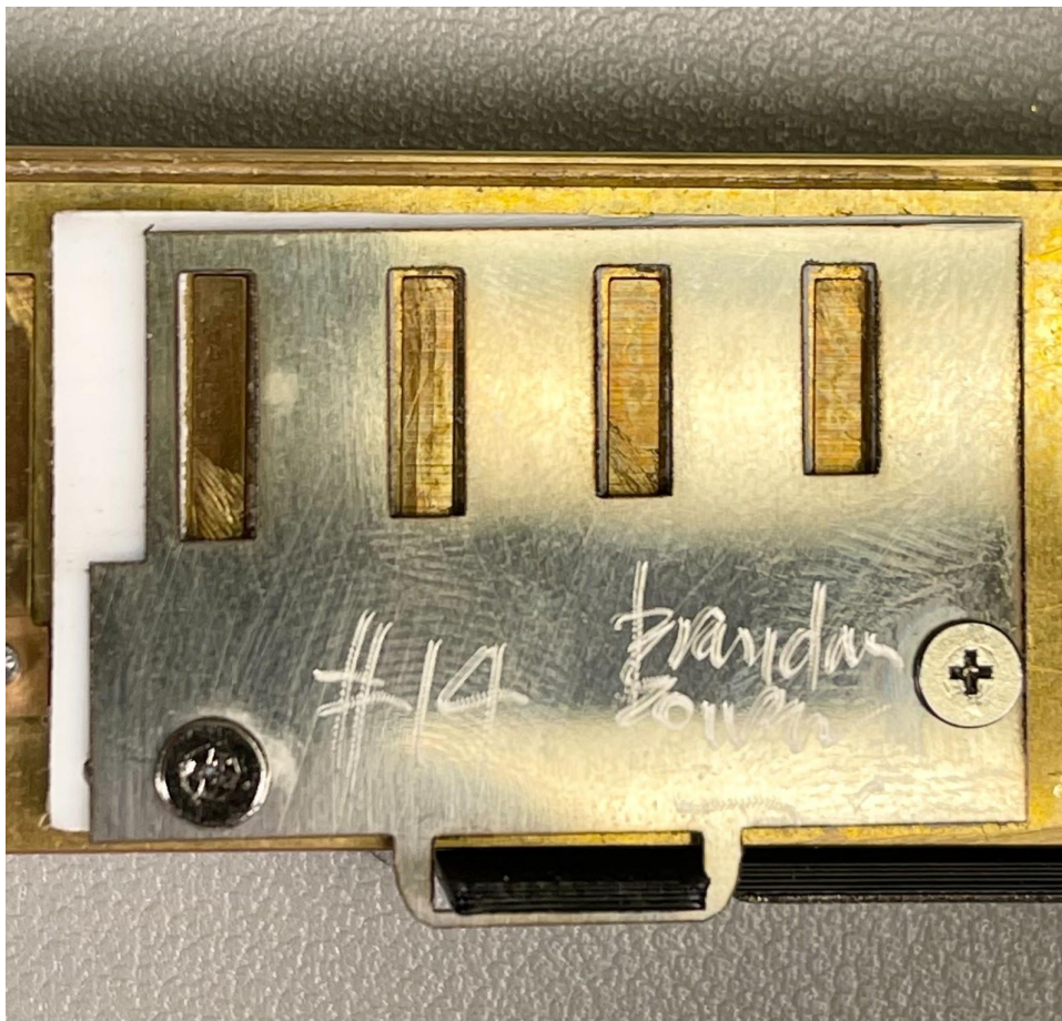
Here is a close-up of the DRAW reed plate side without the slider plate. Easy to see the white Teflon spacer with the precision embedded Neodymium magnets.
