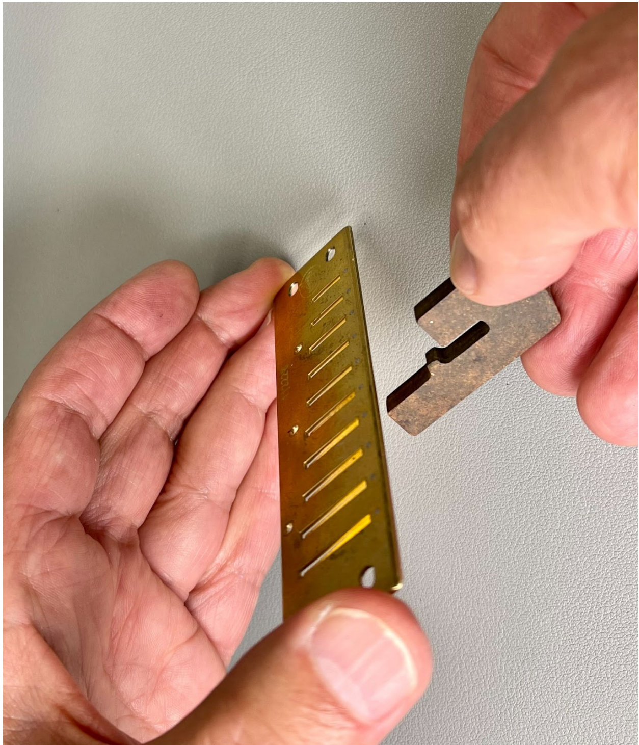
Slide and position the “pin” over the hump of the Reed Plate bow.
