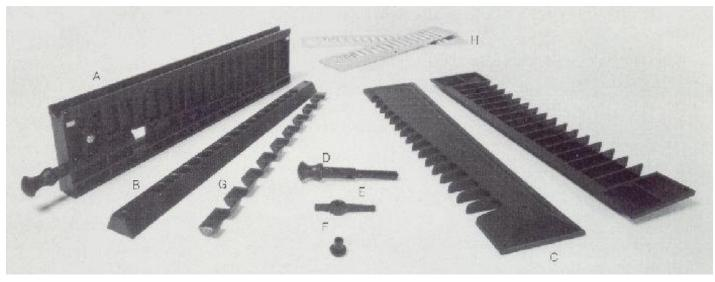
The 32 molded-in chambers -- 16 on each side -- of the "CBH" body or core (A) take advantage of the dimensional stability of glass-filled "Delrin" 570. The contoured mouthpiece (B) and the face plate or combs (C) benefit from its stiffness and smooth, even texture while the slide-actuating plunger (D), lever (E) and bushing (F) utilize its natural lubricity. Slide (G) is molded of "Delrin" AF. Only major use of metal is in the hand-tuned bronze reed plates (H).
