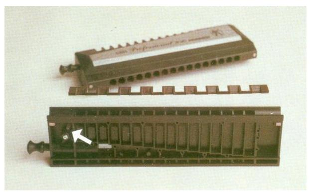
Notched, half-round slide, molded to a tolerance of .001 inch in "Delrin" AF, was designed to glide freely in the groove atop the body of the Hohner "CBH" harmonica, yet eliminate air leakage between chambers. When the spring-return plunger is depressed -- as in the hands of inventor Cham-Ber Huang -- lever (arrow) moves slide to channel air against reeds that sound sharps or flats.
