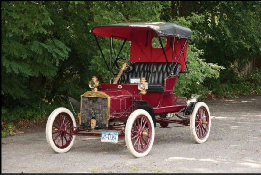
The Ford N was the first automobile to use tough but light vanadium steel. The N also was the car that strived to reach the realm of mass production, though it was still assembled at Piquette with engines and chassis made at other shops.
