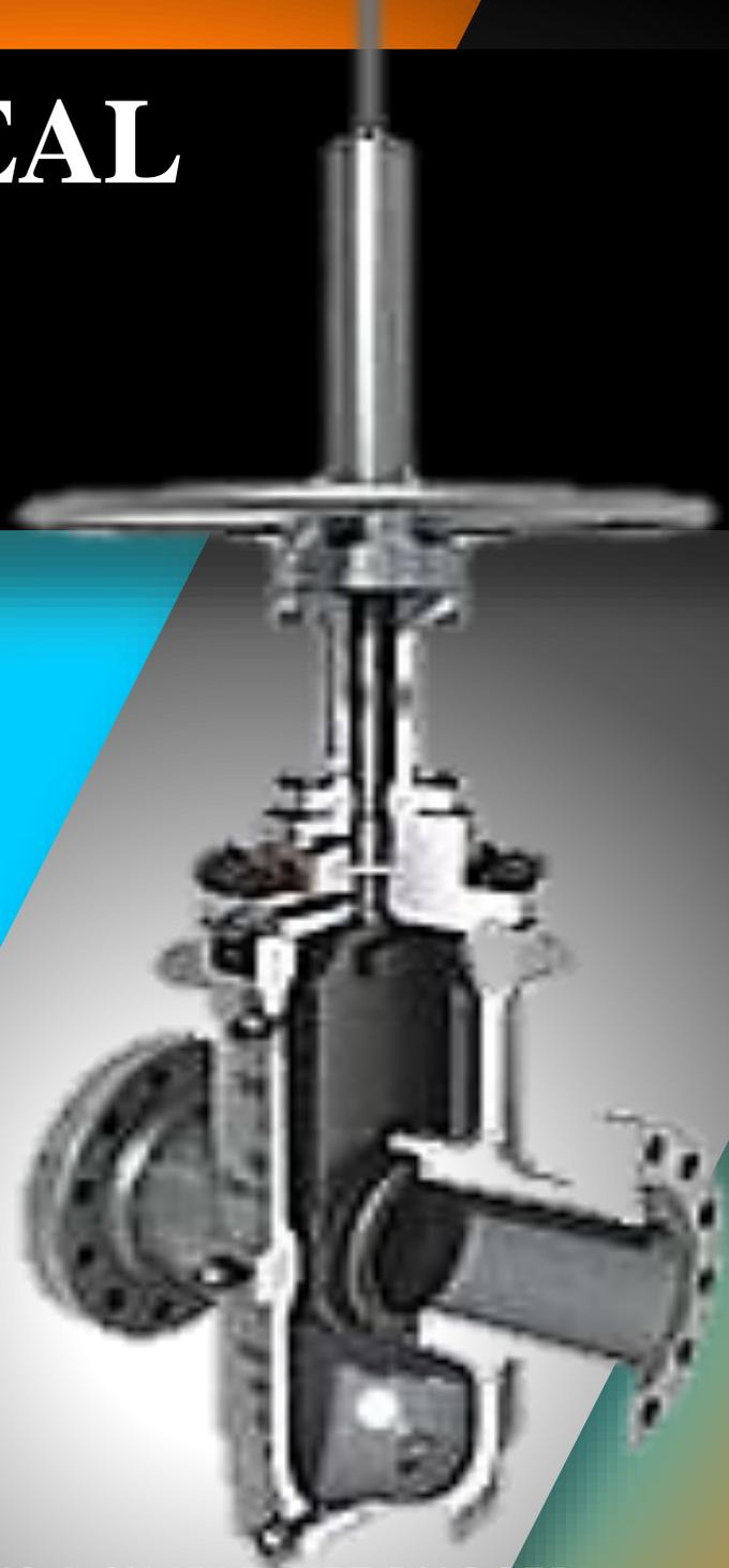
WKM SAF-T-SEAL SLAB GATE VALVE IS A SIMPLE, YET RUGGED AND RELIABLE, THROUGH-CONDUIT VALVE. IT UTILIZES TWO FLOATING SEATS TO PROVIDE A COMPLETE SEAL WITH THE GATE. EACH SEAT CONTAINS A METAL SEAT FACE PLUS A PERIPHERAL SEAL. THE FULL BORE DESIGN HAS THE SAME PRESSURE DROP AS AN EQUIVALENT LENGTH OF PIPE AND ALLOWS PASSAGE OF ALL TYPES OF SCRAPERS (PIGS).
