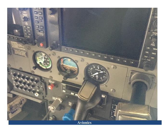
Aircraft is equipped with a G1000 Garmin III Navigation Package, (glass cockpit) which includes:
