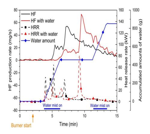
Significant amounts of HF, ranging between 20 and 200 mg/Wh of nominal battery energy capacity, were detected from the burning Li-ion batteries.
