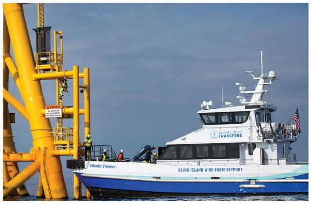
**Figure 3.1-10. Crew Transfer Vessel** *Photograph depicting an example CTV from the Block Island Wind Farm.*
