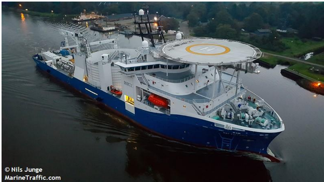
Figure 3.2-5. Cable Lay Vessel Photograph depicting an example cable lay vessel.
