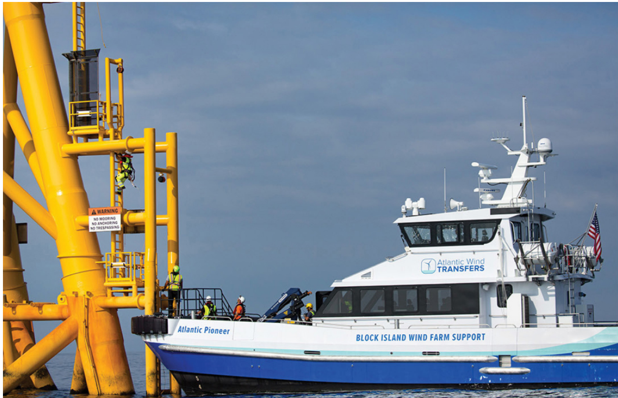
Figure 3.1-7. Crew Transfer Vessel Photograph depicting an example CTV from the Block Island Wind Farm.
