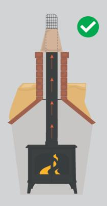
Chimney liners prevent hot fire gasses and sparks from reaching the thatch
