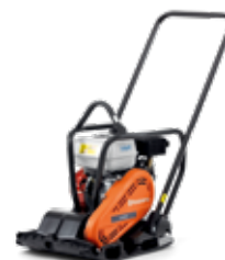
PETROL-POWERED HUSQVARNA LFV 80 3.6 kW, 420 mm, 80 kg, centrifugal force 19 kN.
