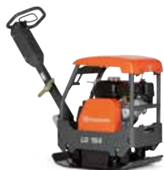
DIESEL-/PETROL-POWERED HUSQVARNA LG 164 3.1–3.6 kW, 148–170 kg, centrifugal force 28 kN.
