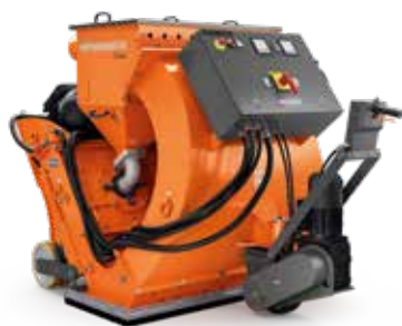
ELECTRIC-POWERED HUSQVARNA BLASTRAC 2-48DS 2×22 kW, 400V, 125A, working speed 0.5–33 m/min, working width 1220 mm, 1350 kg.
