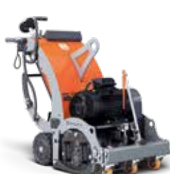
ELECTRIC-POWERED HUSQVARNA BMC 335 16kW, 400V/32-63A, 335mm working width, 430kg.
