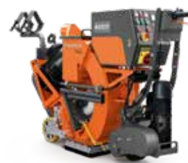
ELECTRIC-POWERED HUSQVARNA BLASTRAC 1-10DS 11 kW, 400V, 32/63A, working speed 0.5–25 m/min, working width 254 mm, 395 kg.
