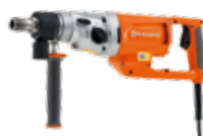
ELECTRIC-POWERED HUSQVARNA DM 210 SP 2000 W, 1-phase, recommended drill diameter 75–150 mm, 6.5 kg.
