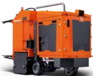
ELECTRIC-POWERED HUSQVARNA BMP 4000RC Remote controlled, 30kW, 400V/63A, 400 mm scarifying width, 380 mm shaving width, 1550kg.
