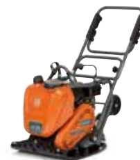
PETROL-POWERED HUSQVARNA LF 75 LAT 3.6 kW, 420–500 mm, 95–97 kg, centrifugal force 15 kN.
