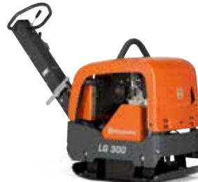
DIESEL-/PETROL-POWERED HUSQVARNA LG 300 4.7–5.3 kW, 265–307 kg, centrifugal force 40 kN.
