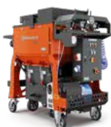
ELECTRIC-POWERED HUSQVARNA BLASTRAC DC 975 7.5kW, 400V, 63A, 510kg.
