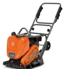
PETROL-POWERED HUSQVARNA LF 80 LAT 3.6 kW, 420 mm, 95 kg, centrifugal force 19 kN.
