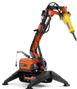
HUSQVARNA DXR 315 27kW, 2020kg, reach 5.5/5.2 m up/forward incl. tool.
