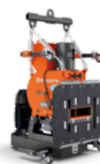
ELECTRIC-POWERED HUSQVARNA BLASTRAC EBE 200V 7.5kW, 400V, 32A, working speed 0.2–20m/min, working width 217mm, 177kg.
