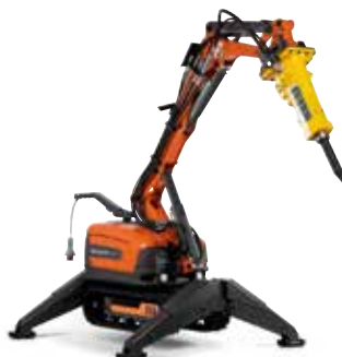
HUSQVARNA DXR 305 27kW, 1960kg, reach 5.2/4.9 m up/forward incl. tool.
