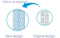
Hydrophilic film fins and inner-threaded copper pipes optimize heat exchange efficiency.
