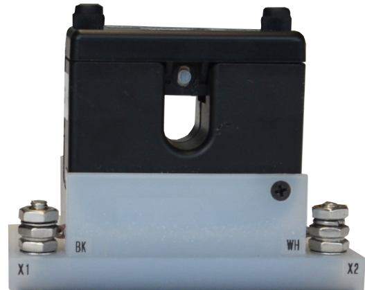
Assembly P/N: APP00849 for 5A=500mV
