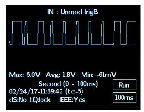
Oscilloscope view and decoded IRIG-B time
