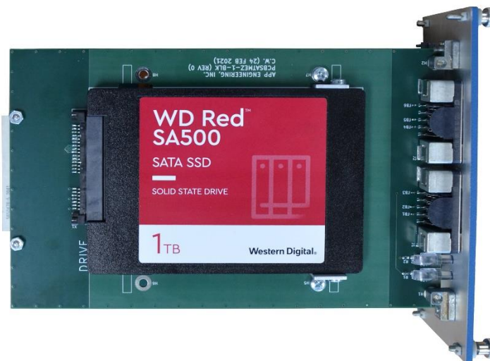
Figure 5 APP 702 Computer Circuit Board with SSD
