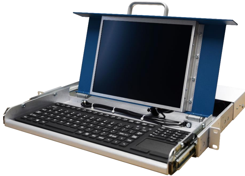
Figure 10 APP-904 Optional Monitor and Keyboard
