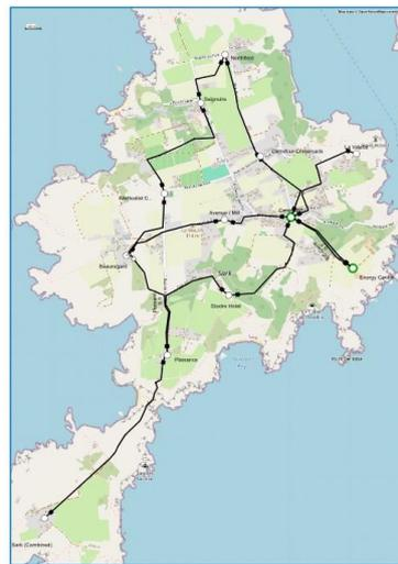
Figure 5-4: Hybrid Design with Central Substation
