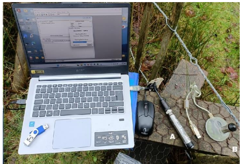
Data collection from a LevelSCOUT (A) and a MiniDIVER (B)
