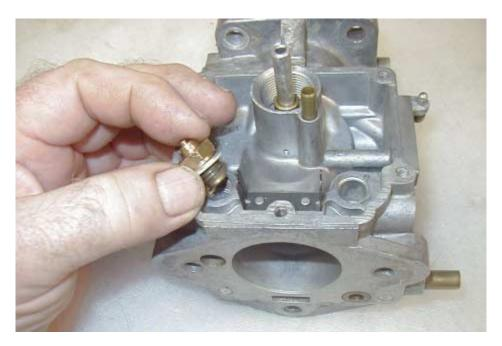
If the valve has been acting up it should be discarded at once lest it end up back in another carb. If the valve is to be reinstalled or kept as an emergency spare, then it should be soaked for an hour or so in the lacquer thinner.
