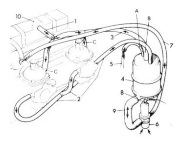
Hoses connect the valve cover (#10) and the canister to ports (C) on the carbs. These hoses are much larger than the ones that connect to the fuel tank and the float chambers. The ports at (C), located above the idle trimming screws, feed directly into the mixing chambers on both carbs.
