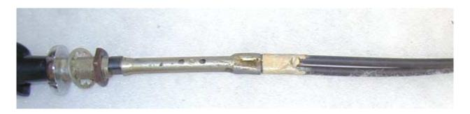
I think this was about the time I bought that new set of carbs that were on the '76 TR6. These carbs have spring loaded cold start valves. I bought the earlier design cable with the flexible inner cable. That was in '84 or '85. It is still working. Moral of the story --- don't try to push a wire.
