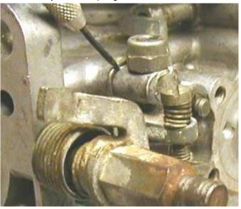
Note the adjustment screw and lock nut to the right of the end of the throttle spring in the adjacent photo. This is the vent lever stop screw. The vent lever is shown in more detail in the next photo. The vent lever is on later carbs, beginning in '73. This venting is discussed at the end of Part I and in the Emissions section next.
