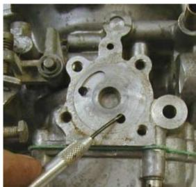
covered and no fuel flows through these passages. When the cold start valve is turned on, a passage is provided between the hole and the slot and fuel is sucked out of the float chamber and into the mixing chamber of the carb.
