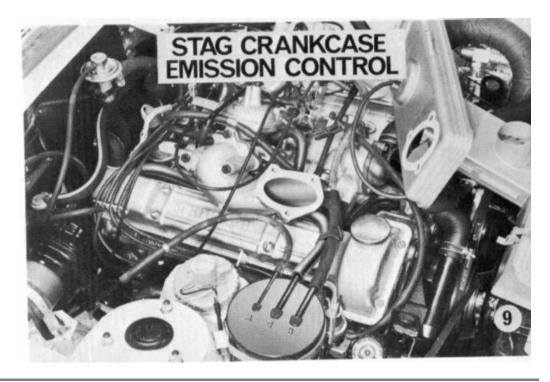
Every 12,000 miles (20000 km) the rocker cover, crankcase emission pipes, tee piece restrictor and purge pipe MUST be cleaned and inspected for deterioration. Renew pipes as necessary.
