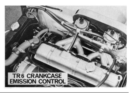
The constant depression is also utilized to cleanse the activated canister of petrol vapour via the purge line which is integrated with the crankcase emission system.
