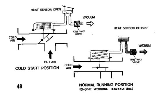
As the engine warms up to normal operating temperature, the sensing device gradually allows the flap valve to accept more air at ambient temperature to provide the correct intake temperature.
