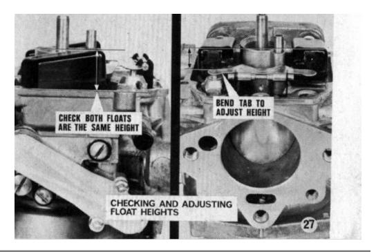
To ensure correct fuel level, check the distance between the float-chamber flange without gasket, to the highest point of each float. Correct measurement 16.0 to 17.0 mm.
