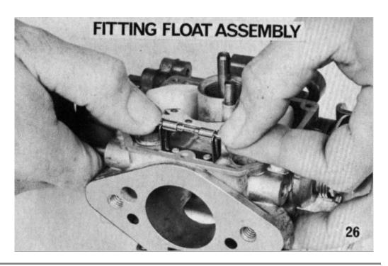
Wash all parts thoroughly and dry with compressed air, NOT RAG. Check the needle valve seating.
