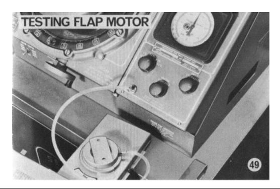
If the action of the air intake control system is suspect through poor cold engine running characteristics, the components may be checked individually as described in the above and succeeding three frames.
