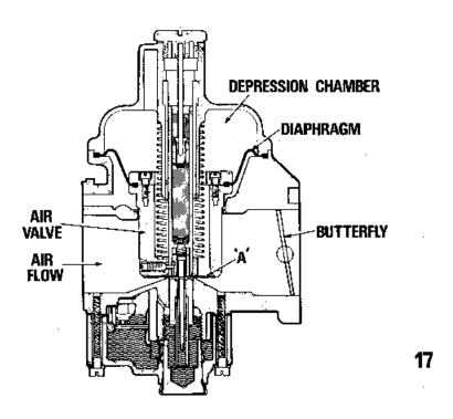
When the throttle is opened, air flow under the air valve increases and a temporary rise in the mixing chamber depression is transferred via drilling 'A' in the air valve to the depression chamber which is sealed from the main body by a diaphragm.
