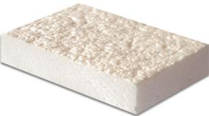
Envirofoam™ TRU-2 is a closed cell, 245fa blown spray polyurethane foam insulation that achieves exceptional yield and adhesion in a wide range of ambient conditions and applications. When applied, Envirofoam™ TRU-2 expands to 25 times its size in approximately 12 seconds to seal and insulate. It can safely be applied in lift thickness of up to 4 inches in a single pass with excellent control and a smooth finish, achieving Appendix X compliance without any additional coatings.
