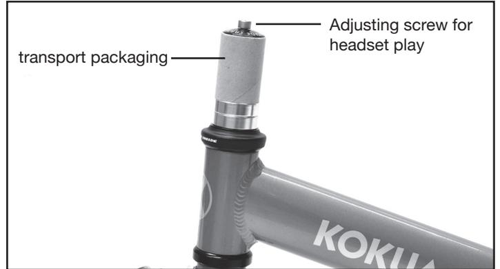
3. Loosen the setscrew adjustment screw and remove the transport packaging.
