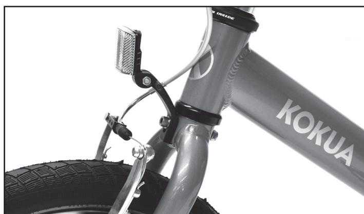
9. The front white reflector is attached to the front fork. Tighten the self-locking nut well!
