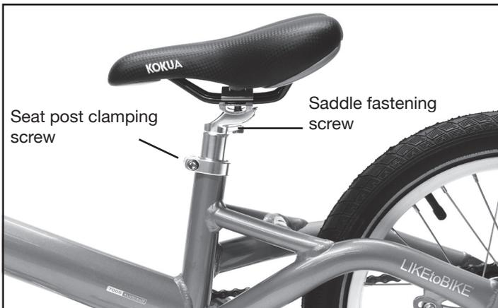
2. After loosening the seat post clamp screw, slide the seat post into the seat tube.
