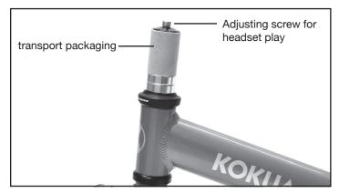
3. Loosen the setscrew adjustment screw and remove the transport packaging.
