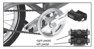
5. Now mount the pedals. Turn the pedal axles by hand until snug! Then tighten with a 15 mm wrench.
