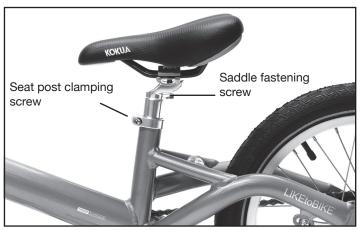
2.After loosening the seat post clamp screw, slide the seat post into the seat tube.
