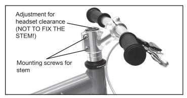
4. Place the stem with the handlebar already mounted on the steerer tube and adjust the headset using the headset adjustment screw.
