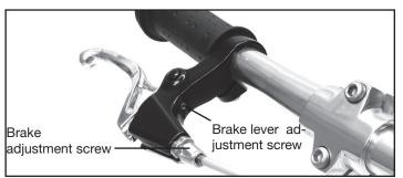
7. The brake lever / handlebar distance can be adjusted to the size of the child with the brake lever adjusting screw. Afterwards the correct distance of the brake pad to the rim may have to be reset! They should be as close as possible to the rim, but not grind.
