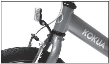
9. The front white reflector is attached to the front fork. Tighten the self-locking nut well!
