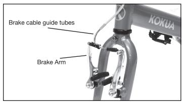
6. To install the front wheel, the front brake must be released. By squeezing the two brake arms, the brake cable can be unhooked by pulling lightly on the brake cable guide tube.
