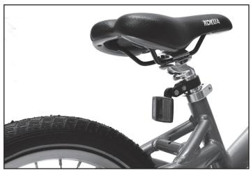
10. The rear reflector is attached to the seat post. The bell is attached either on the right or left of the handlebar
