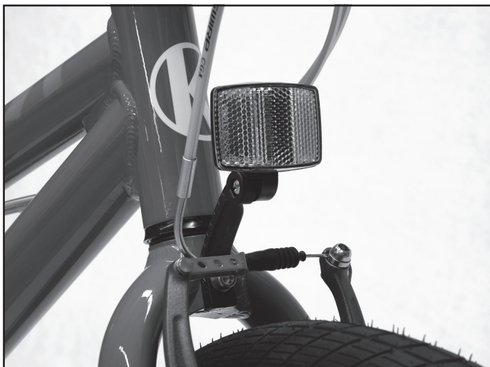
8. The front white reflector is attached to the front fork. Tighten the self-locking nut well!
