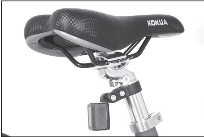
9. The rear reflector is attached to the seat post.
