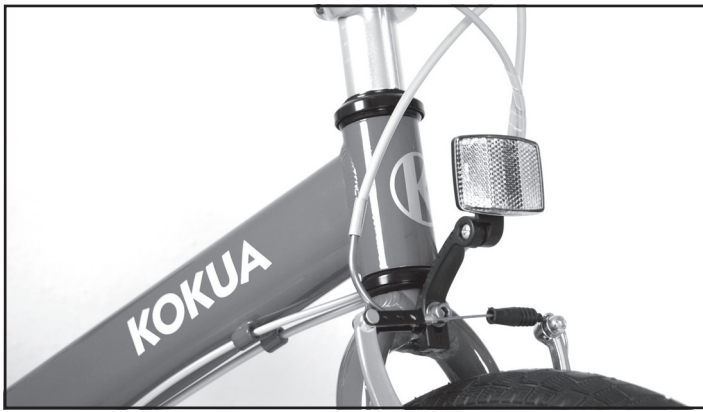
8. The front white reflector is attached to the front fork. Tighten the self-locking nut well!
