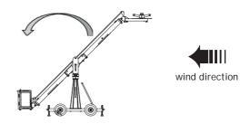
The force exerted on the crane is proportional to the area the wind acts against. Wind blowing from the side "sees" the whole surface area of the boom arm, and may exert a far greater force than if it were blowing parallel to the boom. The wheelbase of the crane might also be narrower in the sideways plane, making overturn more likely in this orientation
