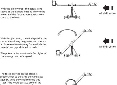
against. Wind blowing from the side "sees" the whole surface area of the boom arm, and may exert a far greater force than if it were blowing parallel to the boom. The wheelbase of the crane might also be narrower in the sideways plane, making overturn more likely in this orientation.
