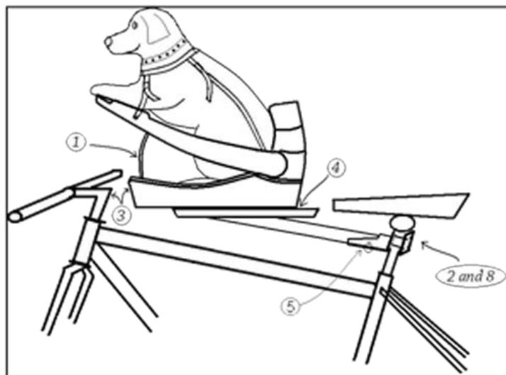
Steps 1 through 7 should never need to be re-done unless the pet seat is mounted on a different size bicycle, in which case the four screws may have to be re-located in different holes to adjust the length.
