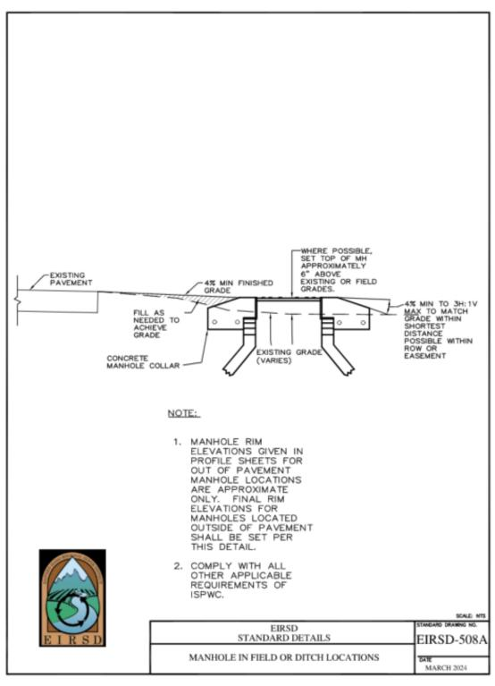
EIRSD-508A (Manhole Collar in Field or Ditch Locations)
