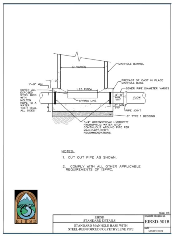
EIRSD-501B (Standard Manhole Base with Steel-Reinforced Polyethylene Pipe)
