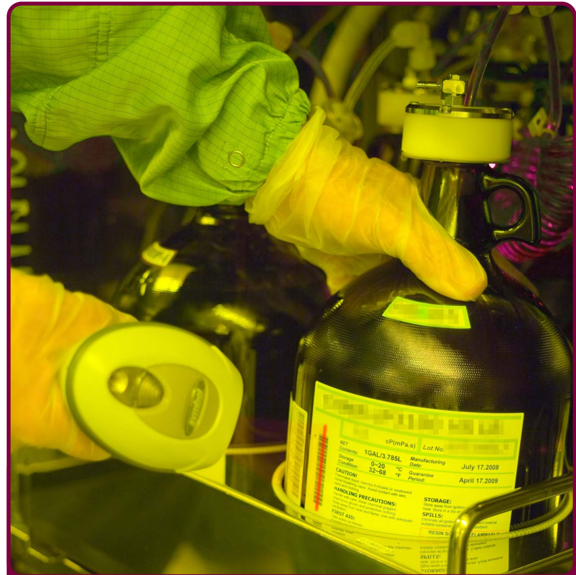
Figure 1. The manufacturer’s bar code and other information is collected and evaluated during a resist change.
