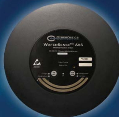
WaferSense Auto Vibration System (AVS) monitors robot health and quality.
