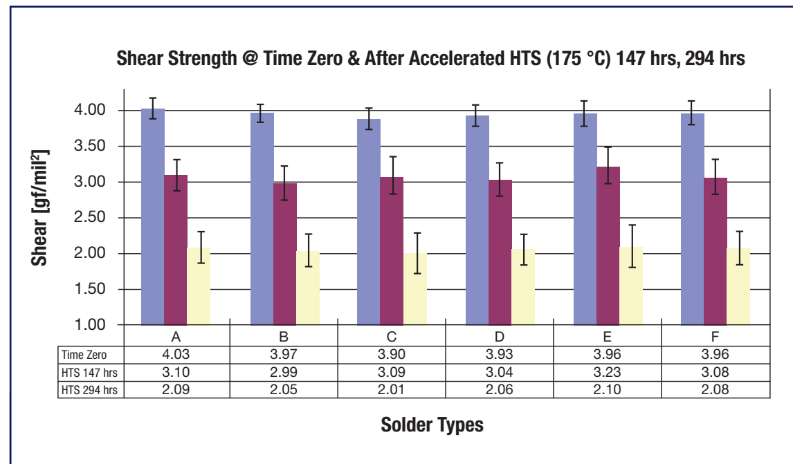
Figure 8. Shear Strength Variation of 6 Types of Solders After High-Temperature Storage
