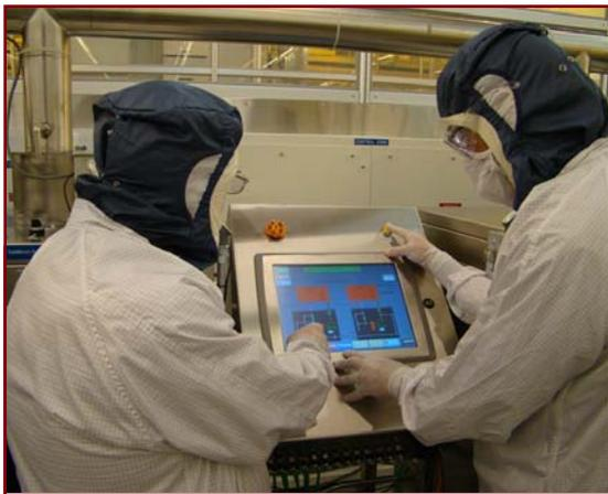
Figure 3. Engineers monitor piping and valve status, I/O signals and alarm conditions through touch screens.
