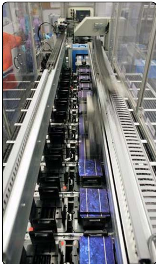
Figure 1 – The PV industry shares many similarities with the semiconductor industry in terms of technology and manufacturing challenges. Shown here are wafer solar cells being sorted at a BP Solar manufacturing facility in 2008.
