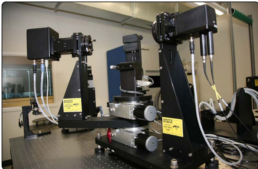
Figure 4 – A dual-rotating compensator ellipsometer in the author's laboratory at the College of Nanoscale Science and Engineering (the RC2™ is manufactured by the J.A. Woollam Company). The modular nature of this and similar ellipsometers makes it highly suited to automated measurement of thickness and optical property uniformity across films on glass substrate used for solar cells.
