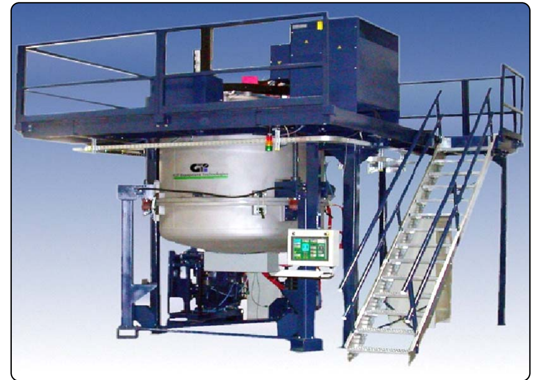
Figure 3 – A typical DSS furnace set up for production of multi-crystalline silicon ingots. This system is bottom loading and components are set up in two levels for better utilization of space.
