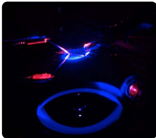
Figure 2 – Small Spot FlashQE Measuring Triple-Junction Cell With Simultaneous Blue and Red DC Bias Lights
