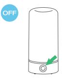
To turn off the AirMoji II, press and hold power button for 3 seconds. The power button light will turn off.
