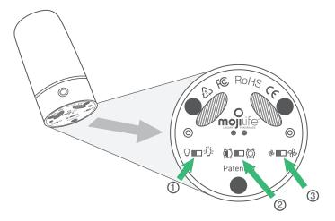
Once the AirMoji II is powered on and in manual mode, you can control the LED light, fan interval, and fan speed settings using the switches located on the bottom of the device.
