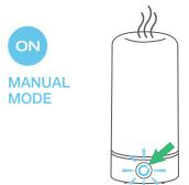
To turn on the AirMoji II, press and hold the power button for **3 seconds**. The power button will light up in blue. Your device is now in MANUAL mode. Instructions for operating
