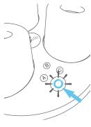
**Step 4:** To activate or deactivate an individual docking port, press the A, B, or C button that corresponds to the desired docking port. This relates to any mode you may have the M3 set in. For example if you are in mode 2 (60 mins off 60 mins on) and have port B deactivated then only A and C will be operating. If you want port B activated you can just simply press the B
