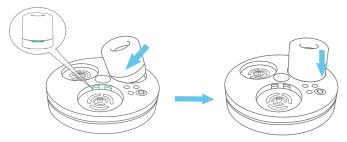
Step 6: Place the three MojiMinis in the docking port on top of the device by inserting the MojiMini at a slight angle and aligning the side notches with the corresponding slots (located toward the center of the M3), once inserted into slot, push down so that MojiMini is flush.
