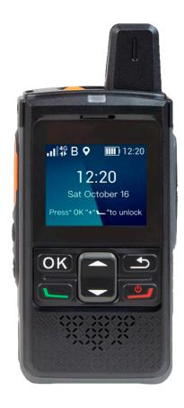
The PNC360s is an ultra-compact, rugged, and easy-to-operate Push-to-Talk over Cellular (PoC) and Wi-Fi device that supports nationwide instant group calling, dispatching, and location tracking.
