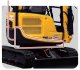
High strength cast iron underside protectors are used to protect the frame corners.
