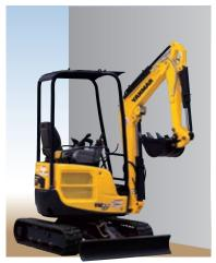
Works efficiently and can be operated without worrying about the tail swing. The excavator body stays within the machine width. This helps reduce the operator's efforts and work time.
