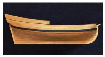
According to the **NRG**, "The purpose of the kit is to teach the novice model builder how to plank a hull the way it was actually done in the shipyard. This process is known as **spiling**."
