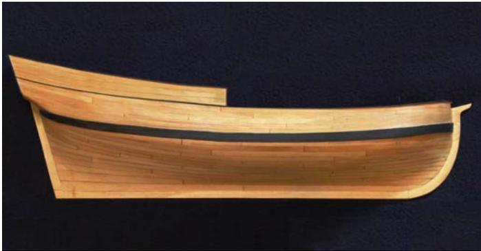
According to the **NRG**, “The purpose of the kit is to teach the novice model builder how to plank a hull the way it was actually done in the shipyard. This process is known as *spiling*.”
