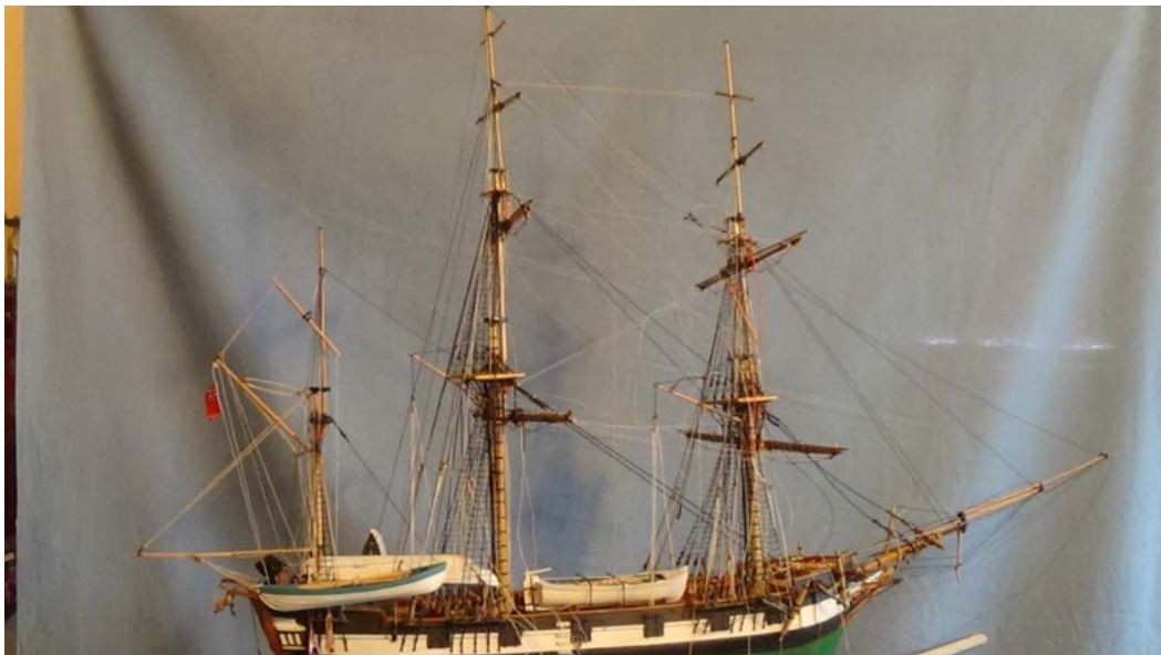
Fig. 9 Partially restored top hamper of HMS Beagle
