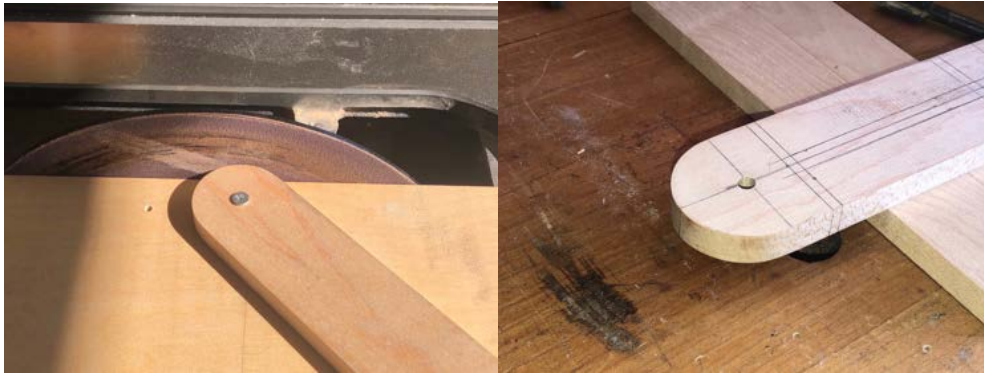
Fig. 18. Making the new carronade base by rotating the end of a piece of maple around a pivot screw against a sanding disk. This gives a perfectly semicircular curve that also has a perfectly orthogonal edge.
