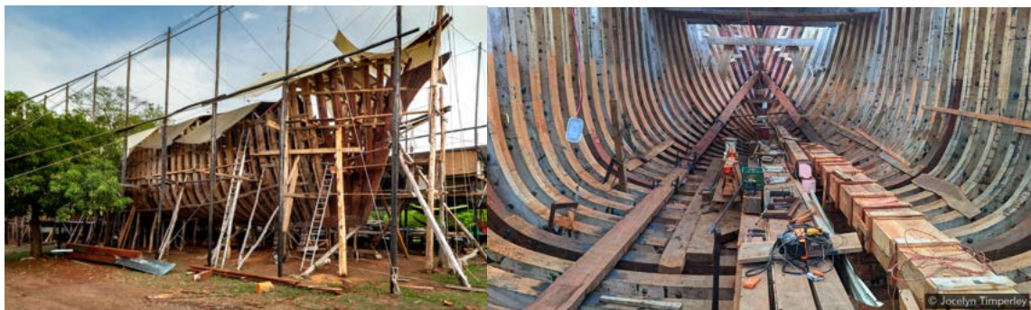
Fig. 3. Wood framing of the Ceiba . (photos courtesy of Sailcargo )
