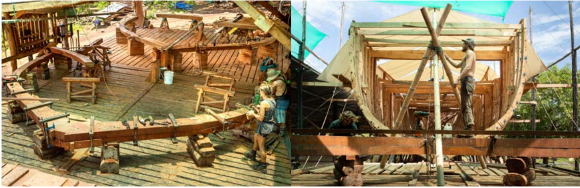
Fig. 4. Wood framing of the Ceiba . (photos courtesy of Sailcargo )
