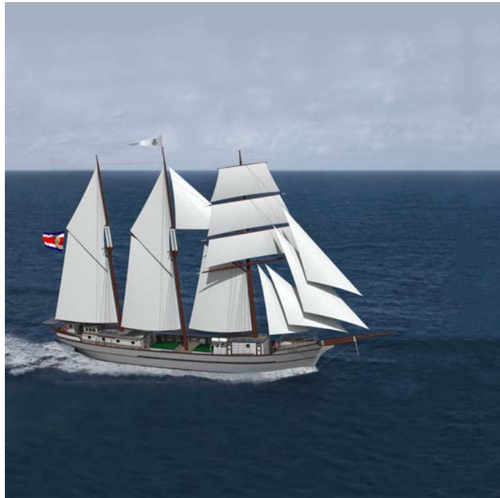
Fig. 2. Proposed electric topsail schooner, Ceiba . (image courtesy of Sailcargo )
