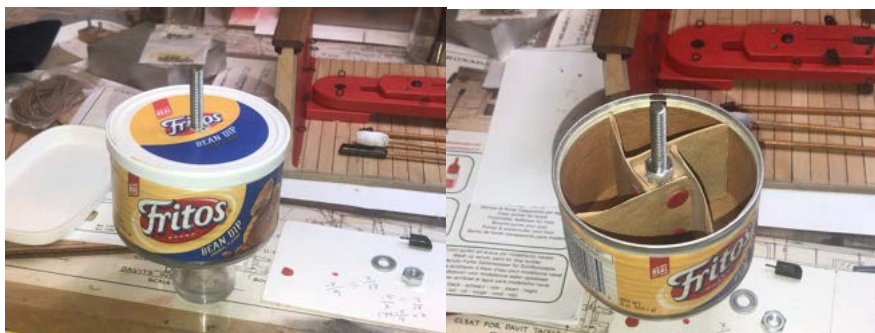
Fig. 7. Home-made block sander made from a bean dip can.
