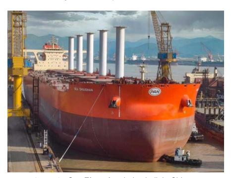
Fig. 2. The **Sea Zhoushan** being built in China with 5 **Norsepower** rotating sails. (Vale)
