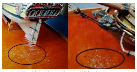
Fig. 6. Exfoliated flakes of material from model fittings found on mounting base.
