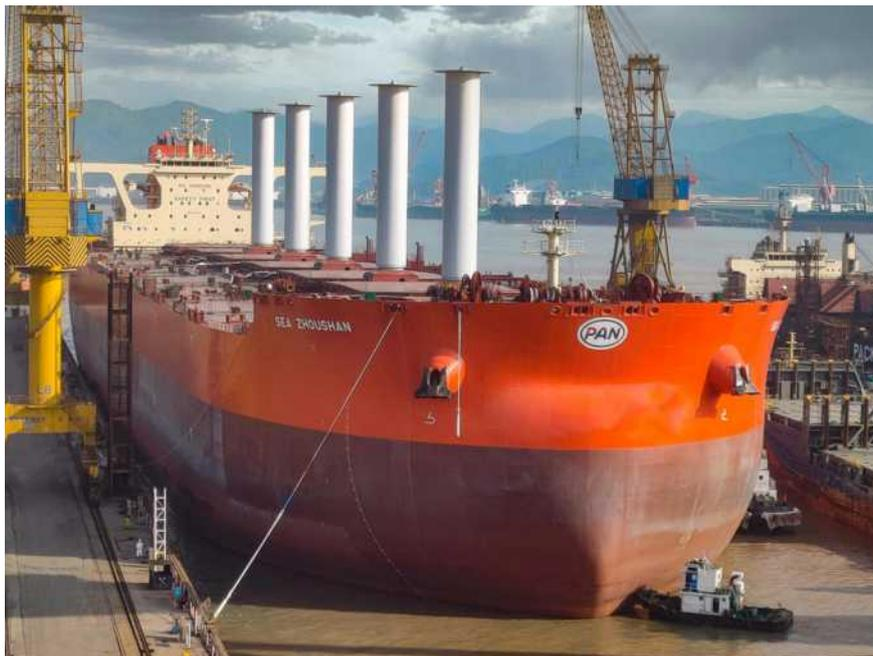
Fig. 2. The **Sea Zhoushan** being built in China with 5 **Norsepower** rotating sails. (Vale)
