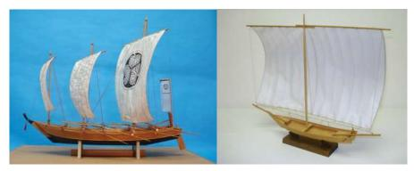
Fig. 3. Two of Clare's models of Japanese coastal boats. Left is a *Hacchoro* boat. Right is a *Hobiki-Bune*
