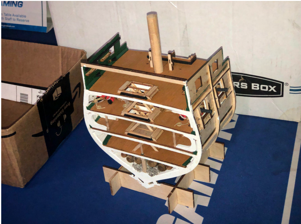
Fig. 12. Jim Tortorici's USS Constitution cross section model with the gunwales now installed.
