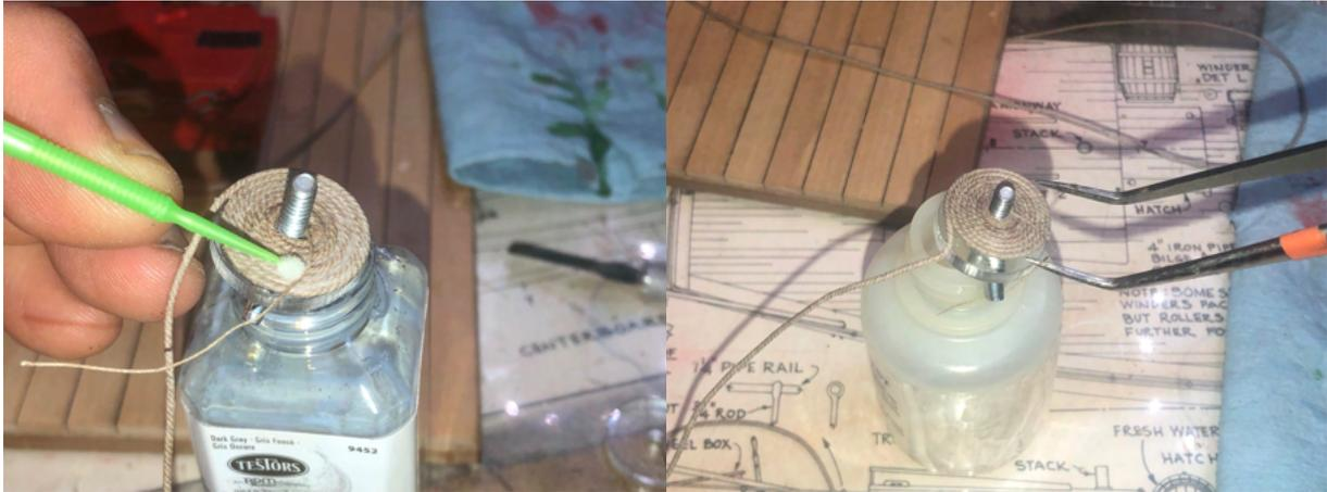
Fig. 10. Left: Applying super glue to reinforce the coil. Right: Lifting the coil off the disk with forceps after the super glue has dried.
