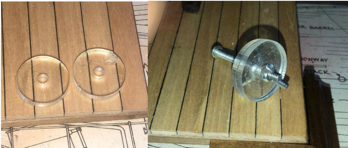
Fig. 7. Jig for making rope coils.
