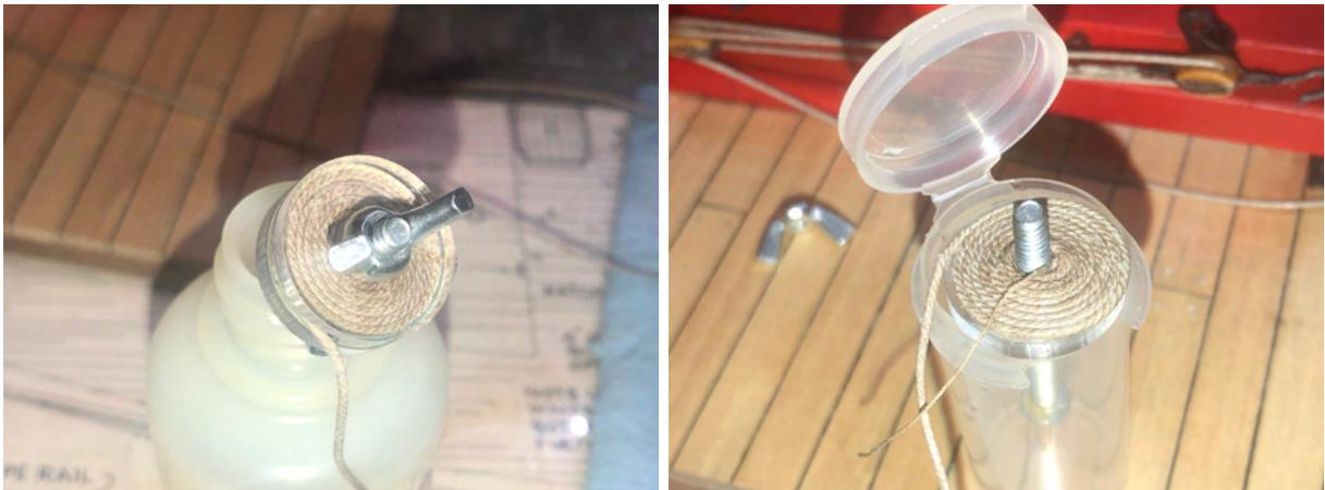
Fig. 9. Left: Winding the rope end into a flat spiral between the disks. Right: Removing the disk on the side of the rope coil that will be glued to the deck.
