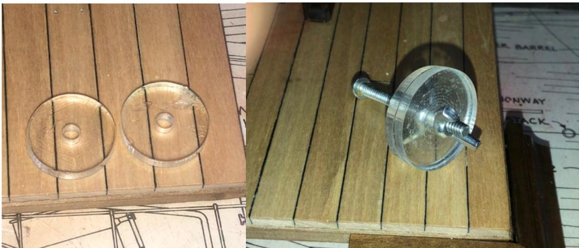
Fig. 7. Jig for making rope coils.
